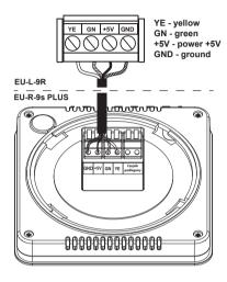
The EU-R-9s Plus regulator can be mounted on the wall. In order to do it, put the rear part of the controller into the flush-mounting box in the wall. Next, insert the regulator and twist it slightly.
