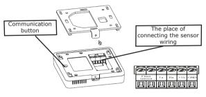
Mount the EU-R-9z sensor hanger on the wall and next fit the cover.
