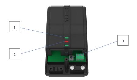
1 – Room regulator status (control light ON - heating). It also signalises communication channel change as described in section III.
